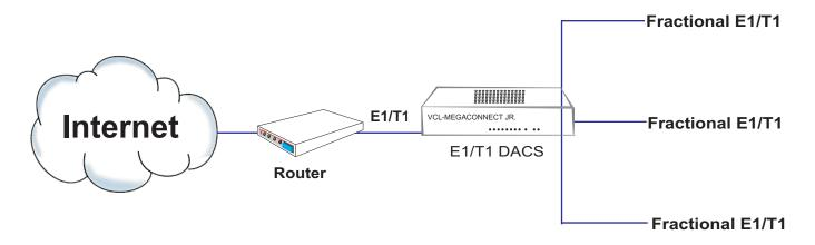
Aggregates multiple E1/T1 Ports to a single E1/T1 Port
