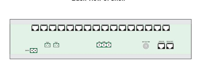
16 Port T1 DACS - VCL-MegaConnect-Jr. Offers programming via an RS232 port for control and monitoring of the unit.
